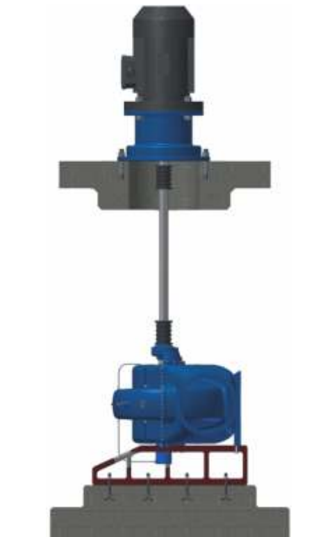
Directly driving of pump by motor with intermediate shaft
