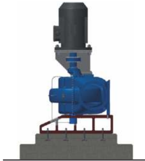
Directly driving of pump by motor
